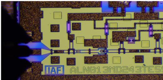
Fig. 14: The test four-stage 325 GHz MMIC. © Fraunhofer IAF
