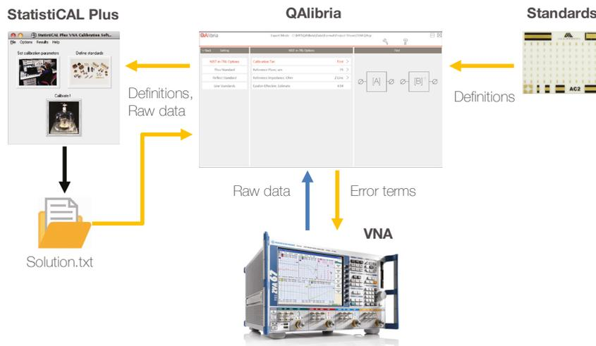
Fig. 7: System calibration data flow.
