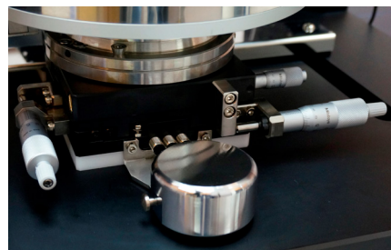
Fig. 7: Air-bearing stage with a single-handed puck control
