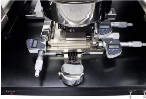
MPI offers the worldwide unique and most accurate contact / over-travel control with 1 µm accuracy for easy measurement reproducibility and accuracy. XY digital micrometers are optionally available as well.
