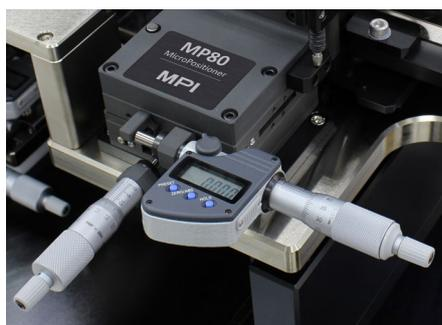
The optional MP80-DX MicroPositioner with the integrated digital micrometer enables outstanding simplicity for the multiline TRL. When operating the MP80-DX, the operator simply needs to zero-out the digital micrometer after the initial adjustment of the probes, i.e., on the thru standard. Next, the distance between RF probes can be easily re-adjusted to the required value of Δl with the precision better than 1 μm.
