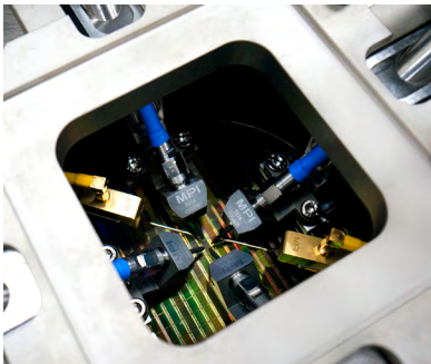
Typical MPI configuration with Kelvin Probes
