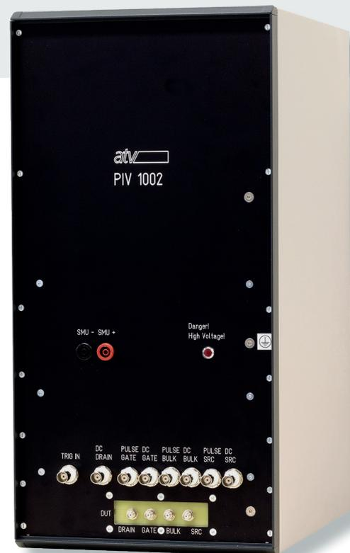
PIV 1002 is a laboratory system for the characterization of high-voltage MOSFET. The system is designed to be carried out on MOSFET pulsed measurements at high voltages and currents. As a result, characteristic curves are recorded without overloading the device thermally.
